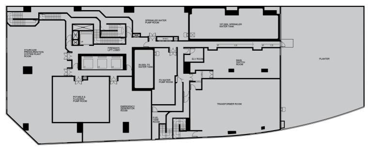
Mechanical Floor at 1/F Floor Plan
